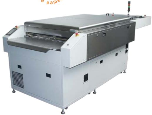
3ES-PROII-WF is designed as inline photopolymer plate washing, rinsing and pre-drying equipment and suitable for processing high quality plates up to a maximum size of 1070 x 1530 mm(42"x60").
